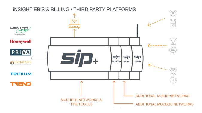
Our solution creates a flexible, multi-protocol integration platform that supports LoRaWAN in addition to all the protocols already available through SIP+ — including Modbus, M-Bus, BACnet, MQTT, REST, and many more.
